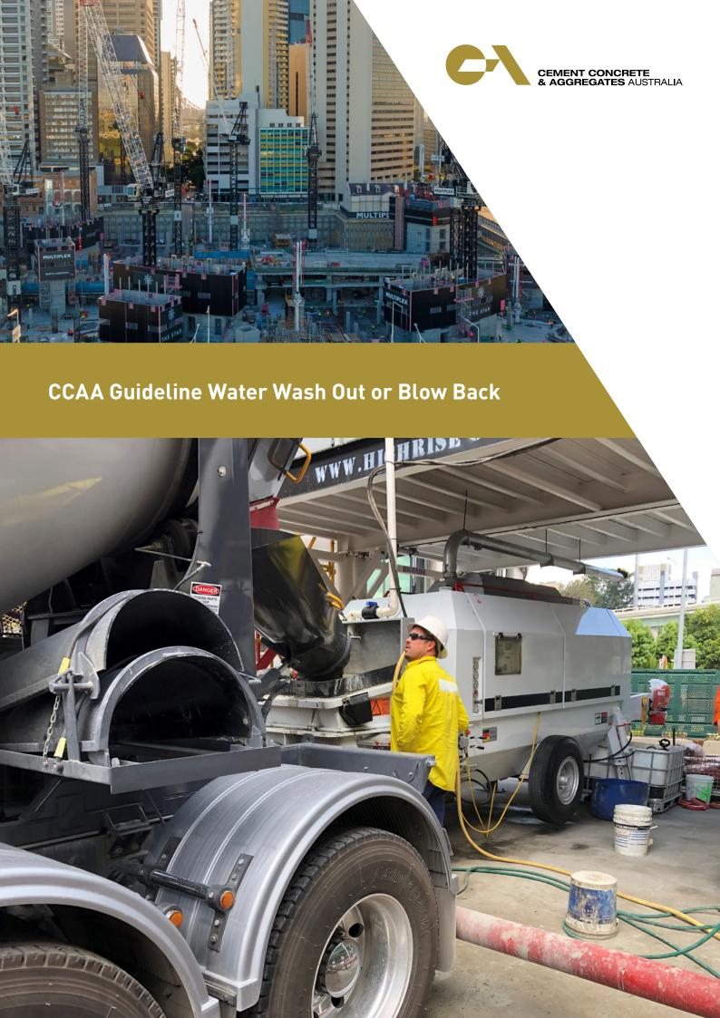
Allowing concrete to be blown back into the agitator barrel is an inherently risky procedure unless it is carefully controlled. Air pressure can cause anything inside the pipeline to act as a high velocity projectile. Water wash out is generally a safer alternative.
